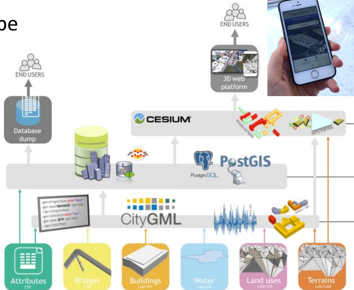
Diagram – Overall architecture of CityGML model's data infrastructure
